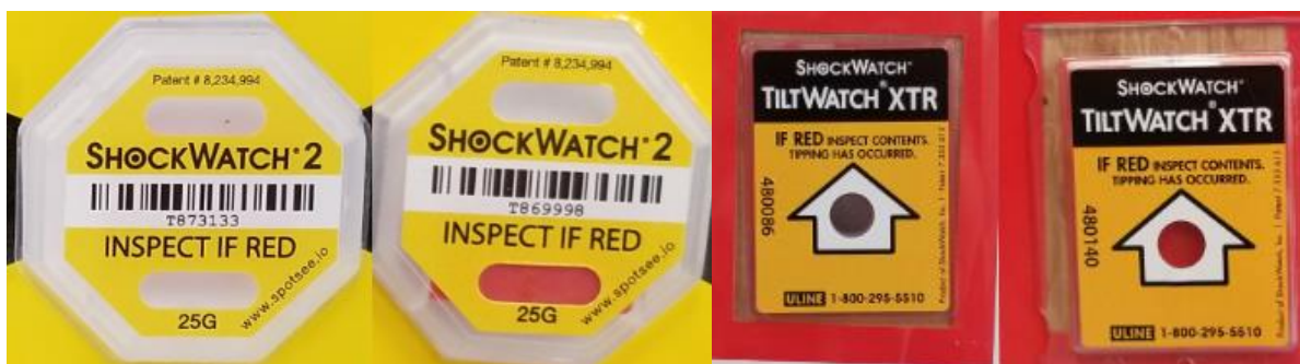
Figure 2: (from left to right) shock-impact sensors (un-triggered and triggered) and tip-tilt sensors (un-triggered and triggered)
