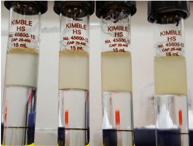
Fig. 4 Density gradient assembly for nuclei purification (Day 1, step 32)
